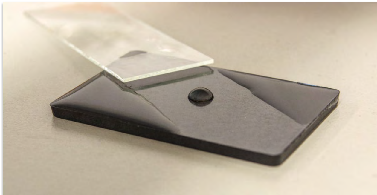
Figure 23: Polyolefin surface still not wettable in the middle due to masking; the drops of fluid remain “sitting”; left and right corners activated and the fluid wets the surface
