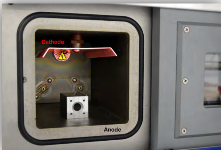
Figure 5: Mounting the substrate on the anode
