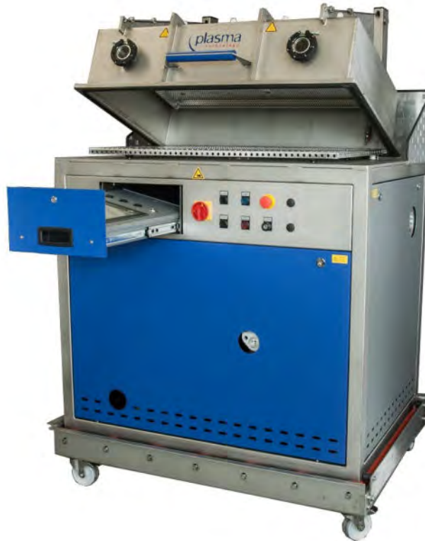
Figure 22: Mobile extraction system designed for removing dust from polymer components
