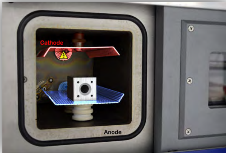
Figure 6: Mounting of the substrate at “floating potential”
