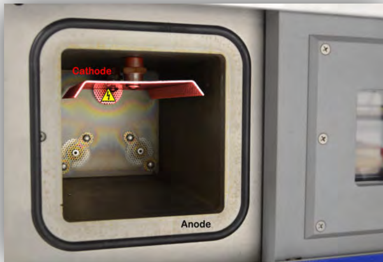
Figure 3: Capacitively coupled LF/HF plasma system, with the chamber wall acting as an anode
