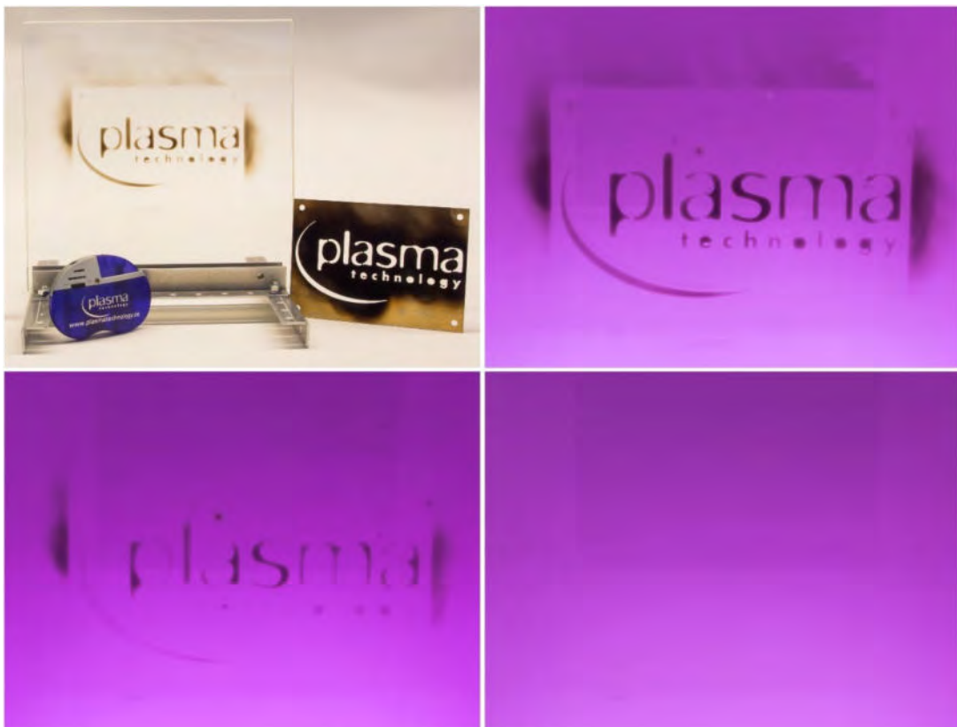
Figure 15: top left: masked glass panel following sooting; View of the plasma chamber during the glass-panel cleaning in low-pressure plasma; top right: Start, lower left: after 60 seconds, lower right - cleaned glass surface after 120 seconds (specified times apply for this cleaning)
