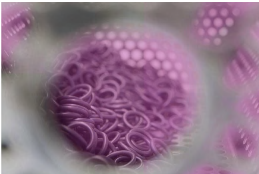
Figure 19: Sealing rings during the cleaning process in a rotating plasma chamber
