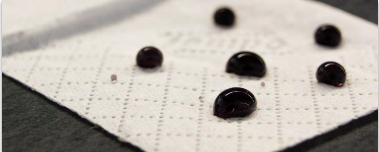
Figure 34: Hydrophobic, non-absorbent surface
