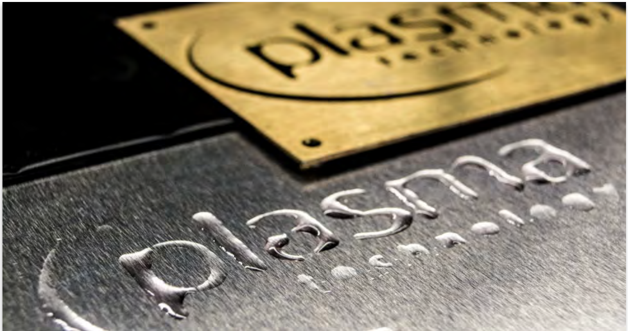
Figure 27: A plasma process carried out with a screen; the lettering clearly shows that delicate, sharply contoured structures can be produced.
