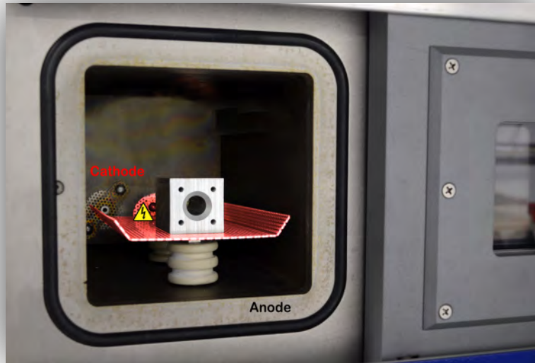
Figure 4: Mounting the substrate on the cathode
